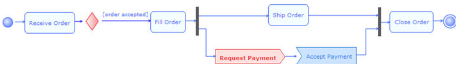
Fig. 10 Conceptual representation (as a UML activity diagram) of an order-to-cash business process, with a syntactic error
