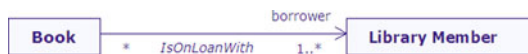
Fig. 11 Conceptual representation (as a UML class diagram) of books on loan with library members that is semantically incorrect
