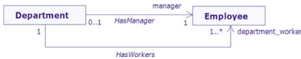
Fig. 13 Conceptual representation (as a UML class diagram) in which being the manager of a department is an optional property of employees
